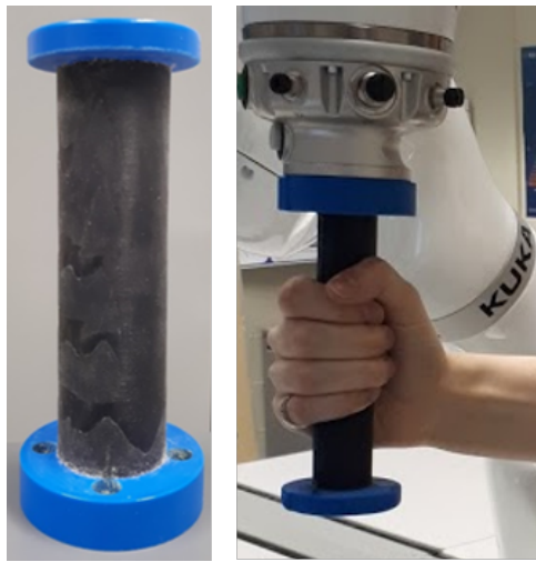
Figure 3.3: First prototype ( Left ), and final design ( Right ) of a handle interface.
